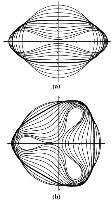
FIG. 4. (a) Numerical solutions of the variational geometric curves with period of  $L_0/2$ . The bold line marks the convex-to-nonconvex transition with the minimum curvature  $K_2 = 0$ . (b) Same as (a) with period of  $L_0/3$ .
